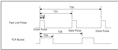
Figure 24. Fast Link Pulse Timing Parameters
